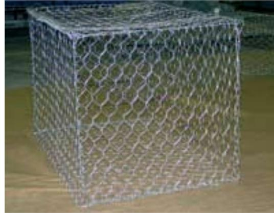
Box-like structures of hexagonal netting with internal partition and a reinforcing board of the following dimensions – length 2 m, width 1 m, height 1 m, the length of reinforcing board – 6 m, made from zinc-coated wire of the 2<sup>nd</sup> class of coating of a diameter of 3.0 mm, with a polymeric coating.
